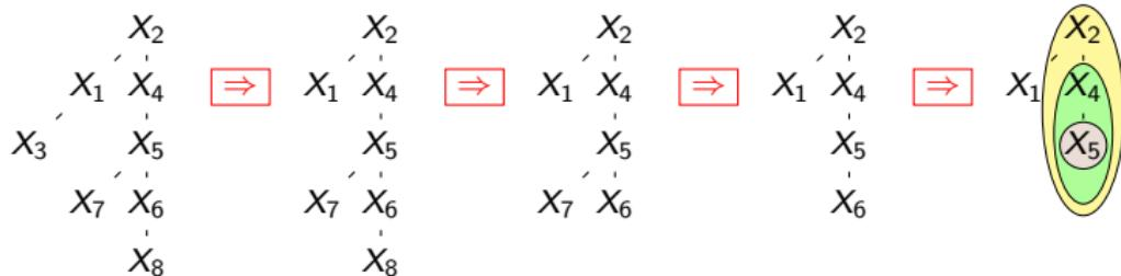
$$\varphi(x_1, x_2, x_4) = \sum_{x_3, x_5, x_6, x_7, x_8} \psi_1(x_1, x_2, x_3) \cdot \psi_2(x_2, x_4, x_5) \cdot \psi_3(x_4, x_5, x_6) \cdot \psi_4(x_6, x_8) \cdot \psi_5(x_5, x_7)$$
