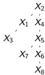
$$\varphi(x_1, x_2, x_4) = \sum_{x_3, x_5, x_6, x_7, x_8} \psi_1(x_1, x_2, x_3) \cdot \psi_2(x_2, x_4, x_5) \cdot \psi_3(x_4, x_5, x_6) \cdot \psi_4(x_6, x_8) \cdot \psi_5(x_5, x_7)$$
