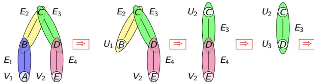
$$U_1(b) = \sum_a V_1(a) \cdot E_1(b, a) \quad U_2(c) = \sum_b E_2(c, b) \cdot U_1(b)$$
