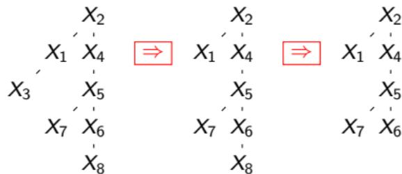
$$\varphi(x_1, x_2, x_4) = \sum_{x_3, x_5, x_6, x_7, x_8} \psi_1(x_1, x_2, x_3) \cdot \psi_2(x_2, x_4, x_5) \cdot \psi_3(x_4, x_5, x_6) \cdot \psi_4(x_6, x_8) \cdot \psi_5(x_5, x_7)$$
