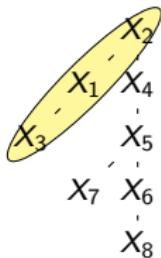
$$\varphi(x_1, x_2, x_4) = \sum_{x_3, x_5, x_6, x_7, x_8} \psi_1(x_1, x_2, x_3) \cdot \psi_2(x_2, x_4, x_5) \cdot \psi_3(x_4, x_5, x_6) \cdot \psi_4(x_6, x_8) \cdot \psi_5(x_5, x_7)$$
