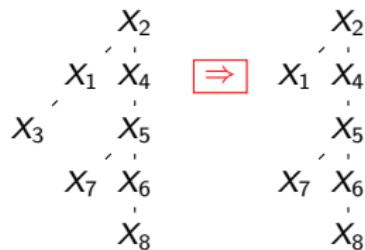
$$\varphi(x_1, x_2, x_4) = \sum_{x_3, x_5, x_6, x_7, x_8} \psi_1(x_1, x_2, x_3) \cdot \psi_2(x_2, x_4, x_5) \cdot \psi_3(x_4, x_5, x_6) \cdot \psi_4(x_6, x_8) \cdot \psi_5(x_5, x_7)$$
