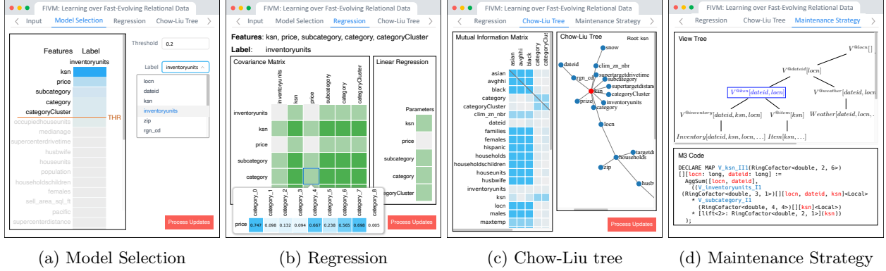
Figure 2: F-IVM’s web user interface: (a) model selection using pairwise mutual information of attributes with a given label; inspect (b) learning the ridge linear regression model with the selected features and label; (c) the mutual information matrix and the Chow-Liu tree; (d) the F-IVM view tree and M3 code for views.
